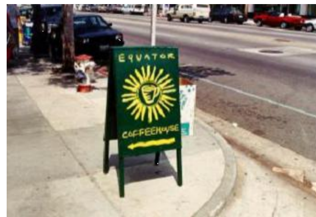
Fig. 14-16: This sign is placed too close to the ADA sidewalk, impeding pedestrian cross walk and access.
